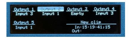
And finally one of the top buttons will be red to show the assigned input of the active output. To change which input is assigned to the active output, simply push on the number of the input that you want to assign it to.
