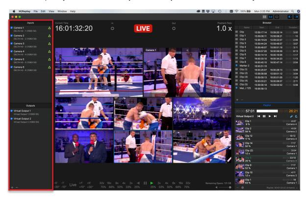
Depending on which video device you use, you will be able to see more or less of them. Note that for some devices (such as with the Decklink Quad 2), if you enable for example the Input 1, you won't be able to enable the corresponding Output 1 as these Inputs or Outputs share the same connector.
