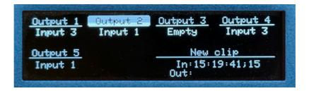
To change the active output with the "Time Spin", hold the SHIFT button down (at the bottom of the vertical NKK buttons), the buttons at the top will be white to show the numbers of output available and the active one will be blue. Just push on the output number you want to select.
